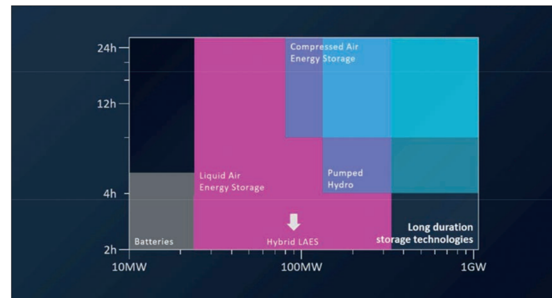
A diagram showing the energy storage options available with their respective storage options – in terms of time and capacity © Highview Power
